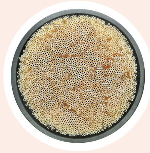
Cross-section of a module containing thousands of membranes
